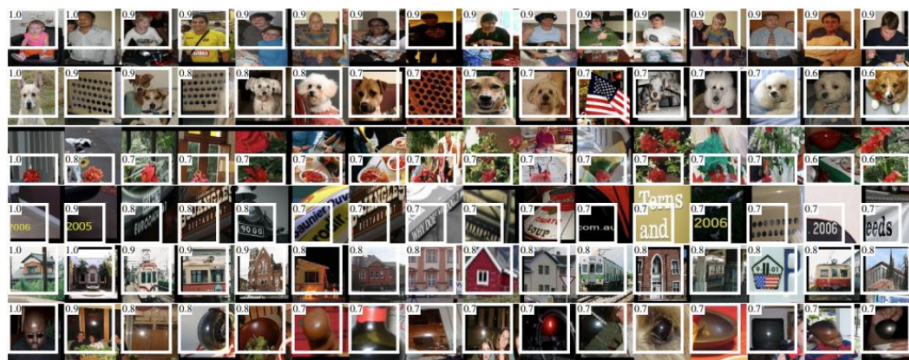
Figure 4: Top regions for six pool 5 units. Receptive fields and activation values are drawn in white. Some units are aligned to concepts, such as people (row 1) or text (4). Other units capture texture and material properties, such as dot arrays (2) and specular reflections (6).
